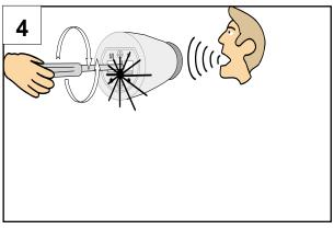
With a small screwdriver, adjust transmitter mic level so the receiver's "AUDIO LEVEL" LED flashes only when speaking very loudly. If it flashes frequently, turn it counterclockwise. If it doesn't flash at all, turn it clockwise.
